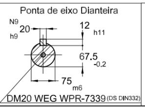
90 kW (125 HP-cv) 04 Polos 60 Hz A
